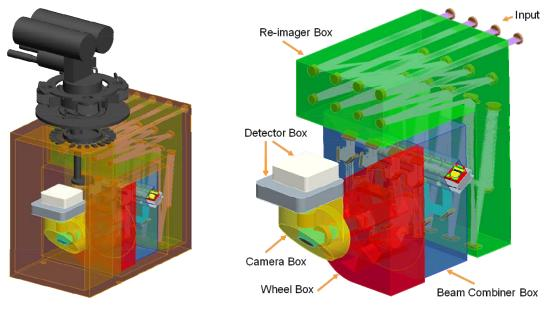
Figure 3: Modular division of the GMA COB concept, backbone and cooler not shown (right)
