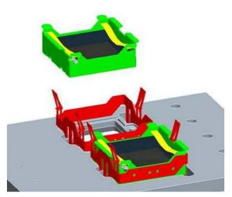
Although not an active mechanism, the mirror clip is an essential COB development. The main purpose of the mirror clip is to provide isostatic mounting of flat optical components (beams splitter/flat mirror) and allow integration on the optical bench single handed, without the use of any tools. The basic idea behind the mirror clip is to reduce the number of parts, risks and time spent on assembly for the large number of small optical elements.
