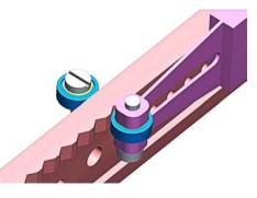
Figure 8: Slit slider indent positioning principle
