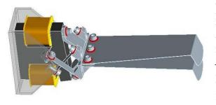
The shutter has two purposes: a light blocking function and a high speed shutter for detector remanence analysis. Providing both functionalities within one mechanism proved impossible so two shutters will be provided. The Cold Shutter is a slow and relative simple type. An off the shelf warm fast shutter is placed just before the entrance window, the side facing the cryostat is gold coated to let the detector look back into the cold environment during a remanence test.
