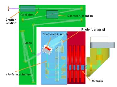
Figure 4: Location of the specific COB mechanisms
