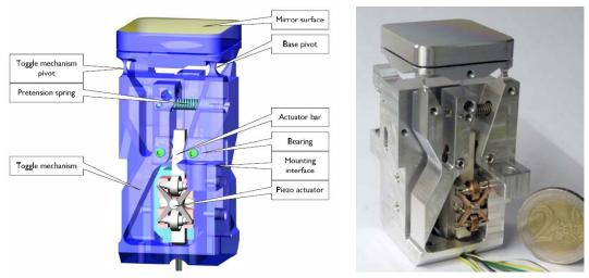
Figure 10 Tip-Tilt Mechanism including piezo motors
